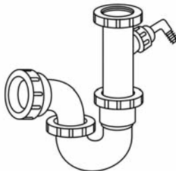
'P' trap with washing machine connection
