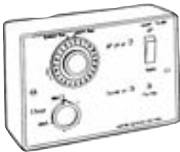
Economy 7 controller for water heater
