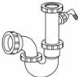
'P' trap with washing machine connection
