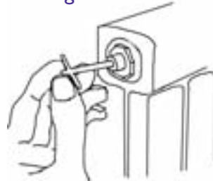
Bleeding a radiator
