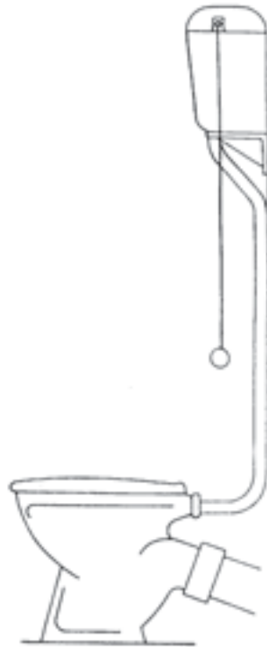
High level cistern
